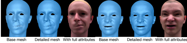
Figure 9: Based on our reliable base meshes, our appearance and detail capture network predicts realistic face skin details and attributes, without special hardware such as Light Stage at test-time, enabling photo-realistic rendering.
